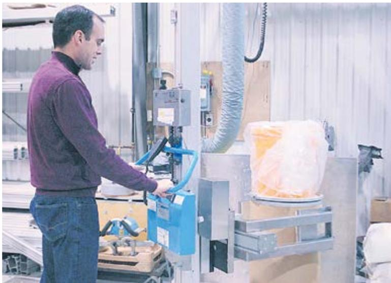
Rob Barrett demonstrates a light-rail barrel lift system. It's a back-saving piece of equipment that requires a single worker to operate it. Photo by Jeffrey Carter
